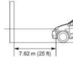
3. **Check the headlights' centerlines** - Pull your car up very close to the garage door, turn on the low beam. Use masking tape to mark the horizontal and vertical centerlines of each headlight on the wall. You'll make three separate markings with the masking tape: Note close up =>
