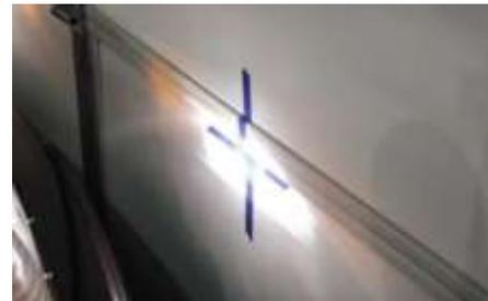
4. **Back the car up, and turn on the headlights** - Back your car so that the front is 25 feet away from the garage door. Turn on the headlight low beam. Check the masking tape marks on the wall to see if the center of the beams match up. Note: Out of alignment =>
