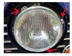
The headlamp is held in place by a captive ring with 3 screws.
