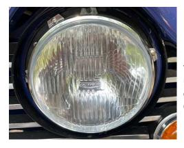
Note: If after installing the captive ring the headlamp is loose, we recommend adding tape or a small piece of gasket material between the ring and the bulb so that when the captive ring is tightened, the bulb is snug. NOTE: DO NOT OVERTIGHTEN.
