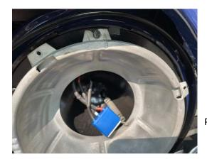
Pull bulb out slightly and disconnect 3 pin electrical plug.
