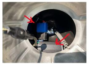
To install new LED headlamps, take the whole assembly and connect the electrical plug. The plug/socket and driver unit should be positioned around the back bottom/side of headlamp bucket.
