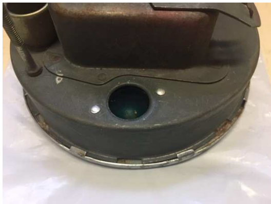
Speedometer/Tachometer with green diffuser
