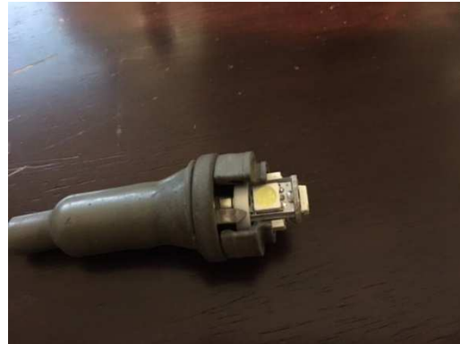
LED in socket with spacer
