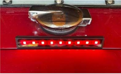
The Auxiliary light can be connected as an additional running light or as a brake light and is designed to fit in the rain gutter of the Triumph TR6 trunk. The light housing is ABS plastic with red lens, a 9 LED strip, double back sticky pads for mounting and approximately 6 ft of two conductor wire terminated for installation.
