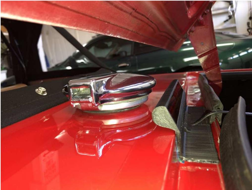
4. If your trunk seal is continuous where the light is, you will need to punch a hole through the seal to feed the electrical wire through into the trunk. We recommend using an upholstery hole puncher. Place the hole just above the stiff portion of the seal. Feed the wire through and into the trunk. If your seal ends join by the light, capture the wire just above the stiff section of the seal so that it is protected from the sharp edge of the trunk gutter. Reinstall the trunk seal.
